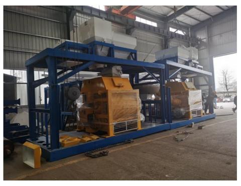
The components of the mixer includes the mixing equipment, driving device, discharging device, charging device, lubricating system,control system and so on.
