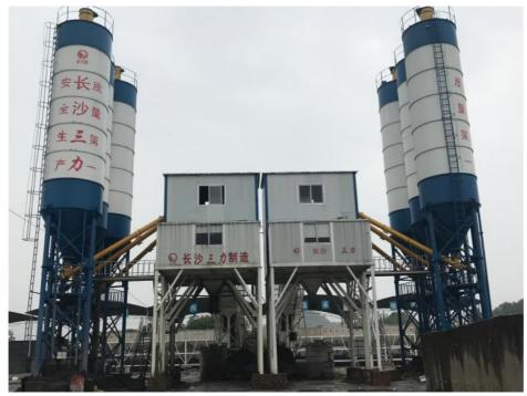
Capacity: The HZS75 model is designed to handle a substantial volume of concrete production. With a capacity to produce 75 cubic meters of concrete per hour, it is well-suited for medium-sized construction projects that require a consistent supply of concrete.
