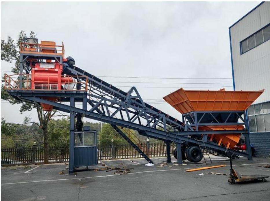
**Mixing Unit:** The YHZS90 features a robust mixing unit, typically incorporating a twin-shaft paddle mixer or a planetary mixer. These mixers deliver efficient and uniform mixing of aggregates, cement, water, and additives, resulting in high-quality concrete with consistent homogeneity.
