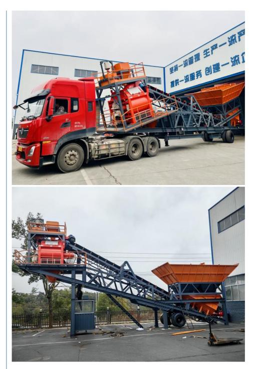
Mobility Features: One of the key features of a mobile batching plant is its mobility. It is designed to be easily transported from one location to another. The plant is mounted on a trailer or a chassis with wheels, allowing it to be towed by a vehicle. Some models may also include folding mechanisms or telescopic legs to facilitate quick setup and dismantling.
